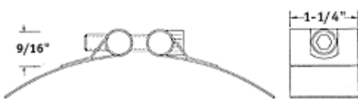
1-1/4" Wide Barrel Assembly Welded to Sheath with 5/16 - 18 socket head screw.
