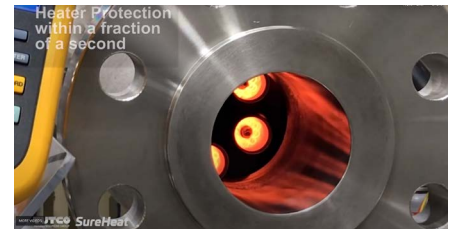
Loss of airflow causes elements to heat up
