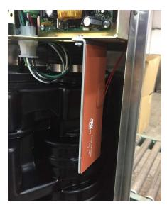
Pneumatic delivery systems use heat for moisture prevention and freeze protection. One of our customers was originally using a screw flange style light bulb before evolving from that solution to a cartridge heater with a unusual bottom that allowed it to be screwed into the light socket. The cartridge heater was very expensive as was the base assembly, and the customer was frustrated with the accelerating cost.
