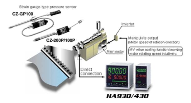
Ultra high speed sampling 0.025 sec The digital PID controller HA930, HA430 realizes 40 times of feedback control in one second and can respond to fast pressure control system of responsibility. Of course we did not speed up only sampling period simply. It should support a high-speed response and, in a setting category of integral value (I) of a PID parameter and derivative (D), is as "0.0 to 3600.0 sec" or "0.00 to 360.00 sec".
