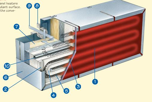
**M E T A L** is the standard face on the M-SERIES panel heaters. The face can be either hard-coated aluminum or porcelanized steel. The remaining construction is exactly the same as the G-Series heaters. The heater face can be provided with air holes for forced airflow as in the FBA construction.
