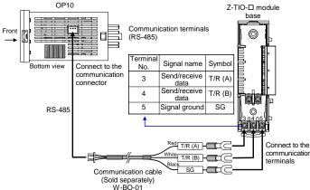
Do not bend the contraction tube section (with termination resistor) of the communication cable. This may damage the cable.
