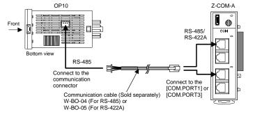
Up to 16 Z-COM-A modules can be connected (however, up to 99 channels)
