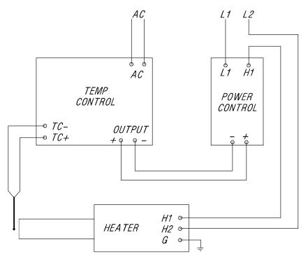
Typical Wiring for 3Ø Heater with Closed Loop Control
