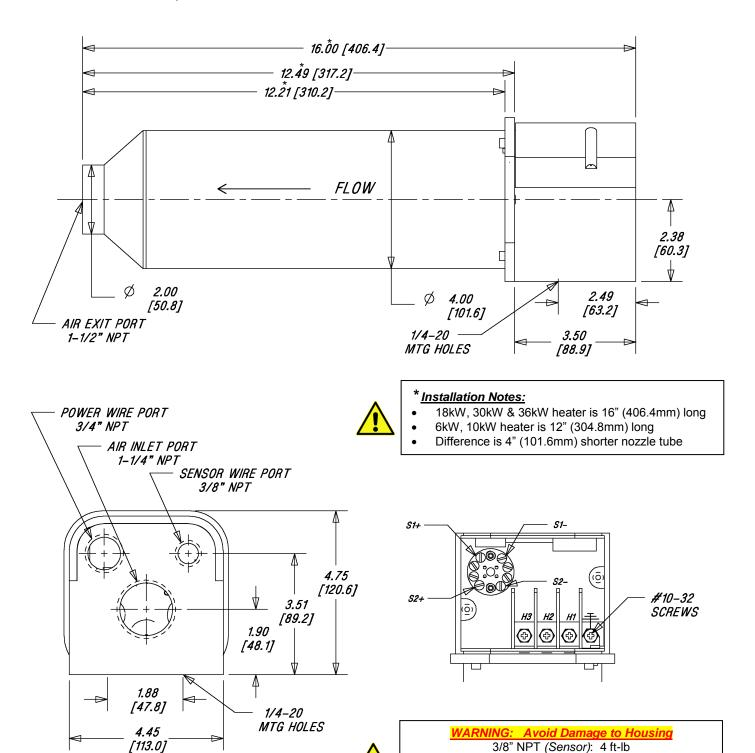
3/4" NPT (Power): 25 ft-lb 1-1/4" NPT (Air): 7 ft-lb (Excessive force will crack housing and void warranty)
