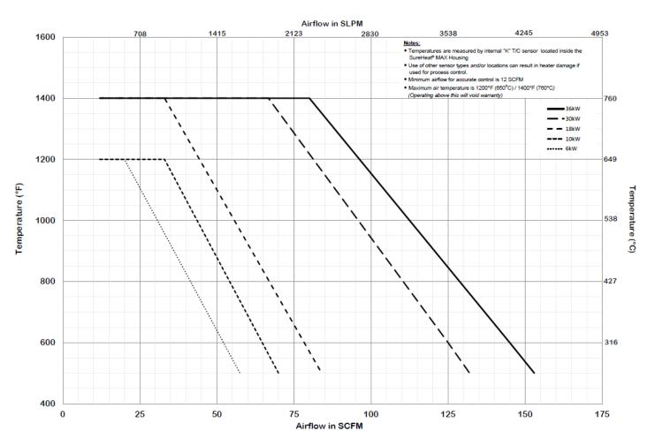
Temperature measured by the internal S2 "K" thermocouple Minimum recommended airflow is 12 SCFM (340 SLPM)
