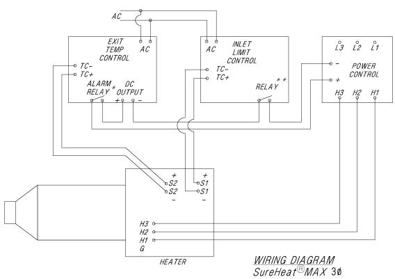
\* EXIT TEMP ALARM RELAY TO OPEN AT 1405°F.
