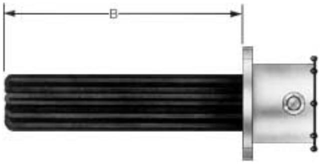
$$B \text{ dim.} = \frac{EHL}{\# \text{elements} \times 2} + \text{cold area}$$
