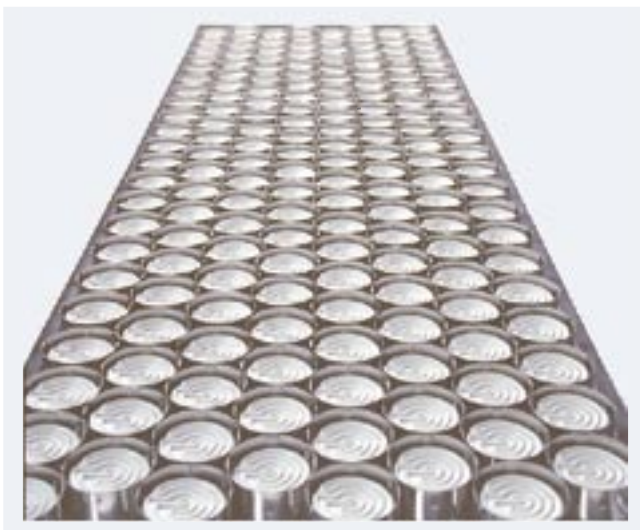
Figure 92: Heating area to heat up the bottoms of bottles
