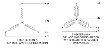
each heater to one of the 3-phase nodes. If you have a multiple of 3 heaters, connect them in equal groupings in parallel. Maybe a few diagrams will help.
