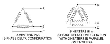
Sparing you the trouble of how to calculate the values, you should read the resistance of one leg divided by 1.5 or R / 1.5 where R is the resistance of one heater when using one heater on each leg. In other words, if you have three  $50\Omega$  heaters connected in a 3-phase delta configuration you should measure  $33.3\Omega$  from A to B, A to C and B to C.
