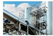
Similar to thermal oxidizers, air scrubbers are designed to eliminate hazardous air pollutants and volatile organic compounds from industrial air streams. The adoption of electric heaters,
