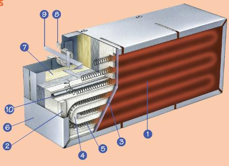
**METAL** is the standard face on the M-SERIES panel heaters. The face can be either hard-coated aluminum or porcelanized steel. The remaining construction is exactly the same as the G-Series heaters. The heater face can be provided with air holes for forced airflow as in the FBA construction. The metal face is used when there is concern of material falling onto the heater face. The metal face is more durable than the glass face. The flip side is that the radiant efficiency
