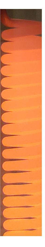
**QUARTZ COMPOSITE** is the standard face on the F-SERIES panel heaters, our best selling heater due to its flexibility, durability, efficiency, and price. It consists of a patented process, using high temperature material, which bonds quartz fabric with a ceramic fiber coil support using a special cement. The end result is a unique, highly durable, quartz composite face heater.
