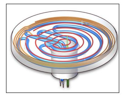
Dual-Zone Cast-In Pedestal with Cable Heaters & Cooling Tube CAS designed and manufactured this pedestal heater using two cable heaters, configured to achieve optimal temperature uniformity. The part also includes a cooling tube and temperature sensors, for easy integration with control systems.
