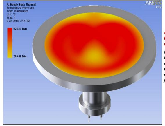
At 624°C, this two-zone pedestal heater has a temperature uniformity of just ±2.3%.
