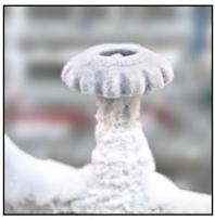
Prevention of J-T Cooling, Icing Installing a CAST-X Heater in-line warms expanding gases to prevent valve and component freezing.
