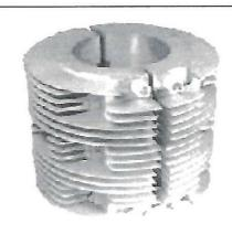
Air-cooled heaters feature a variety of cast fin patterns to circulate forced air across the body of the casting. Specific fin patterns are used to maximize this airflow for efficient process cooling of the extruder barrel. Low profile fin patterns can be used for areas with restricted space or rapid cooling requirements. In some cases, the cooling capacity of the air-cooled design can be augmented with cast-in cooling tubes to maximize the cooling function.
