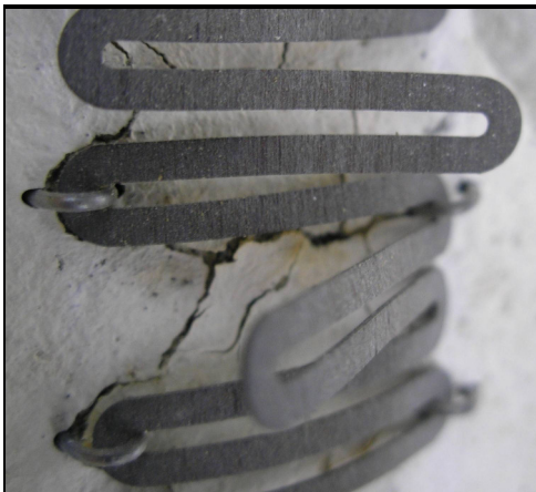
Close-up of pinned elements after high temperature cycling. (Note cracks in the refractory board)
