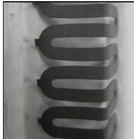
Close-up of V-series after high temperature cycling (No cracks in refractory)
