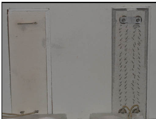
Back side of heaters during test V-series on left. pinned elements on right
